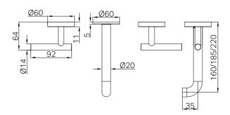
Compatible with bodies 25D016 (centre spout position) and 25D017 (offset spout position).
