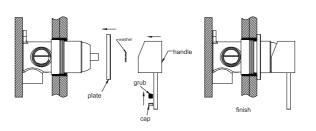
10. Slide plate onto body, attach the washer to the cartridge, position the handle, tighten it with a grub screw using an Allen key, and cap the grub screw hole.
