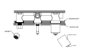
4. Remove the gauge, self-tapping screw, washer, and plastic sleeve in sequence.
