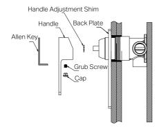
6. Install the back plate against the wall. Fit the handle adjustment shim onto the cartridge stem, attach the handle using a grub screw, and cover the grub screw hole with the cap.
