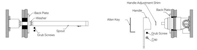
6. Install the back plate on both sides against the wall. Fit the handle adjustment shim onto the cartridge stem, attach the handle using a grub screw, and cover the grub screw hole with the cap.
