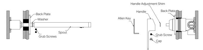
6. Install the back plate against the wall. Fit the handle adjustment shim onto the cartridge stem, attach the handle using a grub screw, and cover the grub screw hole with the cap.
