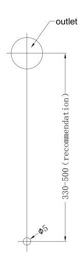
1.Drill a φ6mm hole at the outlet vertical downward position in the recommended range.
