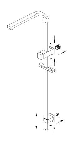
4. Adjust lower body position, and put diverter body and lower body on to the outlet adapter and the bracket, then tighten grub screws by Allen key.
