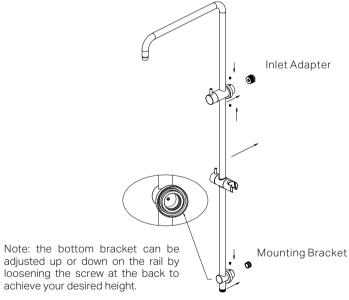
4. Position the shower rail assembly over the wall adaptors. Adjust the position of the bottom bracket to align with the mounting holes on the wall
