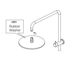
5. Screw the overhead shower into the shower arm, ensuring a rubber washer is in place for watertight seal.
