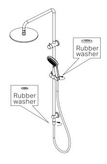
6. Attach the hand shower to the hose and connect the hose to the shower rail, ensuring that rubber washers are in place at both connection points to prevent leaks.
