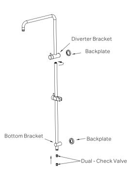
1. The recommended height for the water outlet is 1653-1753mm from the finished floor surface.
