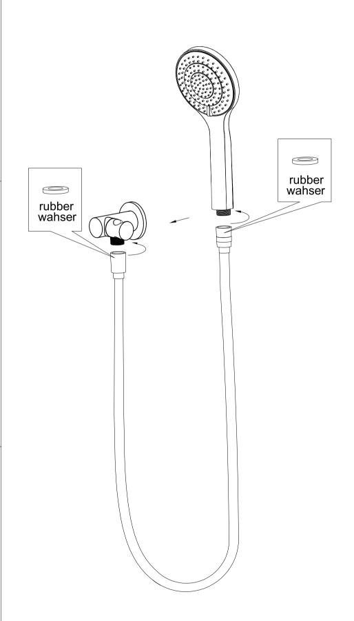
4. Connect bracket and hand shower with hose. TEST & CHECK FOR LEAKS.
