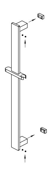
6. Install shower rail onto brackets, tighten four grub screws by hex wrench.
