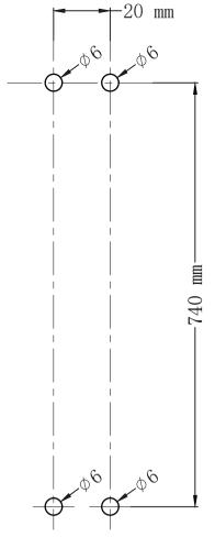
4. Drill four holes according to above picture.
