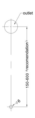
1.Drill a φ6mm hole at the downwards outlet vertical downward position in the recomendation range.
