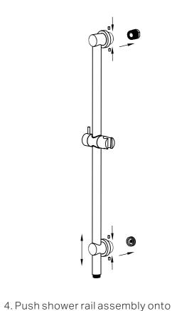
the wall/tile face. Tighten grub screws firmly. Slide the back plates against the wall/tile face properly.
