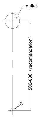
1. Drill a p6mm hole at the downwardsoutlet vertical downward positionin the recomendation range.
