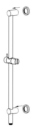
3. Slide both top and bottom back plate onto the rail assembly, as shown on the picture.
