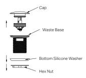
01. Remove the cap, hex nut, and bottom silicone washer from the waste base.
