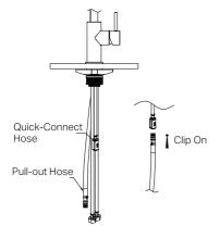
04. Connect the pull-out hose to the quick-connect hose.
