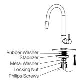
03. Slide the rubber washer (stabilizer if needed) and metal washer over the threaded tube, secure the mixer firmly to the benchtop with locking nut and Philips screws.
