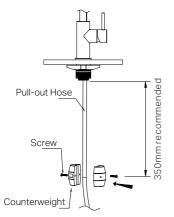
05. Install the counterweight onto the pull-out hose using the screws provided. It is recommended to position the counterweight approximately 350mm below the base of the mixer
