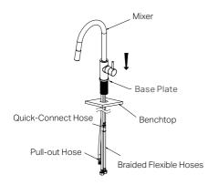
02. Place the mixer body on the benchtop, with the quick-connect hose and braided flexible hoses passing through the hole in the benchtop.
