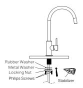
3. From underneath the benchtop, compress the rubber washer and metal washer against the base using the locking nut(if a stabilizer is required, install the stabilizer after positioning the rubber washer), then tighten the Phillips screws to secure the mixer.
