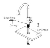
2. Pass the flexible hoses through the hole on the benchtop from above, then place the mixer body onto the benchtop. Ensure the O-ring is fitted inside the base ring and sits flush around the hole for a proper seal.
