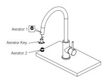
Note: Use the aerator key to remove and replace the aerator as needed.
