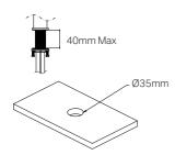
1. Pre-drill or create a hole with a diameter of 35mm at the proper location. Please note that the thickness of the surface should be between 3mm-40mm.
