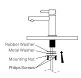
3. From underneath the benchtop, compress the rubber washer and metal washer against the base using the mounting nut, then tighten the Phillips screws to secure the mixer.
