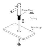
2. Pass the flexible hoses through the hole on the benchtop from above, then place the mixer body onto the benchtop. Ensure the O-ring is fitted inside the base ring and sits flush around the hole for a proper seal.
