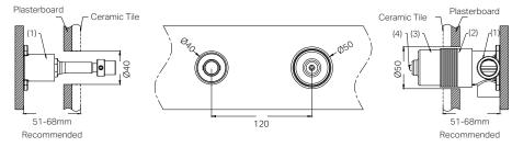
1. Secure the mixer body (1) to the nogging, ensuring an installation depth of 51-68mm from the nogging to
