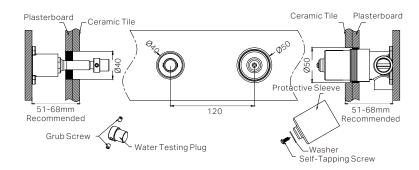
1. Drill a ø50mm and a ø40mm hole in the ceramic tile, then position it as shown in the above diagram. 2. Undo the self-taping screw to remove the protective sleeve, and release the grub screws to remove the water testing plug.
