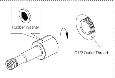
3. Attach the G1/2 spout adapter to the outlet thread, ensuring that the rubber washer is properly seated inside the adapter as illustrated in the figure.
