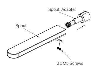
2. Unscrew the 2 x M5 screws, and then remove the G1/2  $\,$  spout adapter from the spout.
