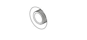
1. Trim the G1/2 outlet thread to be flush with the finished wall surface.
