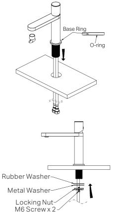
2. Place the mixer body and pass the Pex hoses through the hole in the counter-top. Ensuring the O-ring sits within the bottom groove of the base plate to prevent water leakage through the cabinet.
