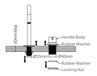
4. Insert the handle body through the Ø40 mm hole(ensure the rubber washer is positioned between the handle and benchtop).
