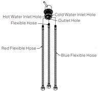
5. Install the three different flexible hoses into the corresponding holes on the handle body as shown in the diagram. Red-H, Blue-C
