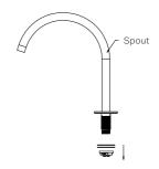
2. Remove the locking nut, metal washer, and rubber washer from the spout.
