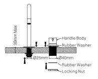
4. Insert the handle body through the Ø40 mm hole(ensure the rubber washer is positioned between the handle and benchtop).
