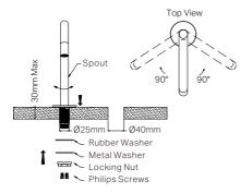
3. Rotate the spout to the midpoint of its 180° swivel range.
