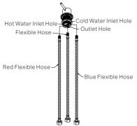
5. Install the three different flexible hoses into the corresponding holes on the handle body as shown in the diagram. Red-H, Blue-
