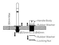
4. Insert the handle body through the Ø40 mm hole(ensure the rubber washer is positioned between the handle and benchtop).
