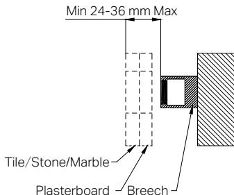
1. Before installation, ensure the distance between the breech face and the finished tile/stone/marble wall surface is 24-36mm.
