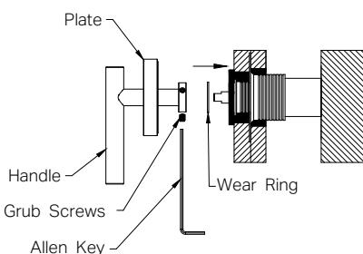
13. Slide the wear rings onto the spindle connections.
