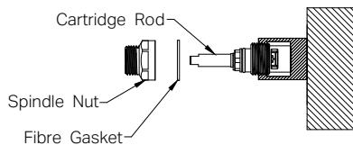
2. Tighten the cartridge rods firmly into the in-wall breech with a torque wrench.
