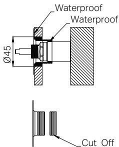
5. Install the plasterboard, and drill two Ø45mm mounting holes at the designated location.
