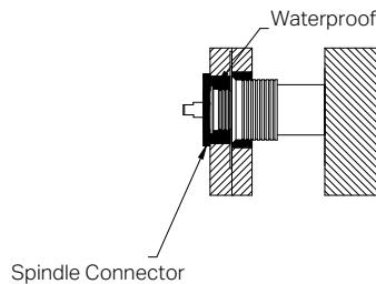
9. Screw the spindle connectors onto the spindle nuts and measure the length protruding beyond the finished tile/stone/marble wall surface.
