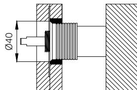
8. Install the tile/stone/ marble, and drill two Ø40mm mounting holes at the designated location.
