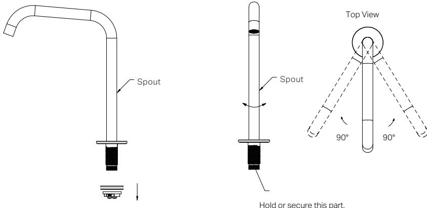
2. Remove the locking nut, metal washer, and rubber washer from the spout.
