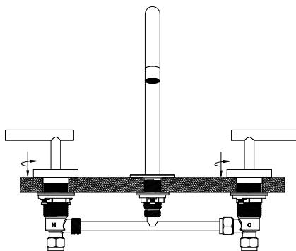
8. Slide the plates down to cover the fittings and tighten them in place.
