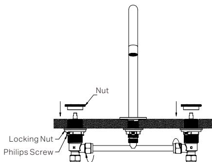
6. Push-fit the T-piece into the spout, and align the valves with the two mounting holes. Ensuring the body sets sit flush. Hand-tighten the nuts onto both valve bodies. Secure the body sets with locking nuts, then further secure them with Phillips screws. Tighten the hex nuts on both ends of the T-piece to prevent leaks.
