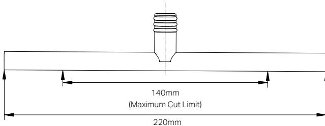
1. Cut three holes on the benchtop as shown in the diagram:
