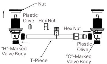
5. Identify the hot(H) and cold(C) valve body. Unscrew the nuts on the top, and hex nuts, plastic olives on the sides from valve bodies. Fit the plastic olive and hex nut onto the T-piece on both sides, slightly tighten the hex nuts. Do not overtighten to allow for later alignment.
