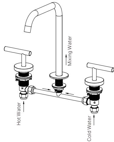
9. Turn on the water supply and check all connections for leaks.
