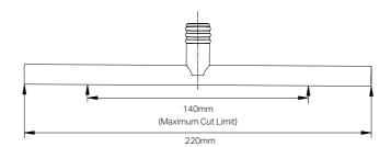
1. Cut three holes on the benchtop as shown in the diagram:
