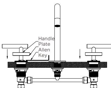
7. Slide the plates up and fit the handles onto the spindles. Tighten the grub screws with an Allen Key.
