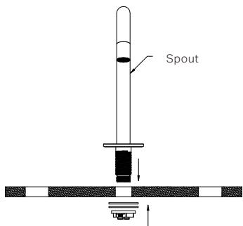
4. Insert the adjusted spout into the centre hole.
