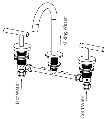
9. Turn on the water supply and check all connections for leaks.
