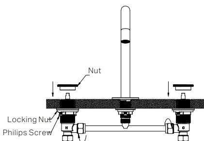
6. Push-fit the T-piece into the spout, and align the valves with the two mounting holes. Ensuring the body sets sit flush. Hand-tighten the nuts onto both valve bodies. Secure the body sets with locking nuts, then further secure them with Phillips screws. Tighten the hex nuts on both ends of the T-piece to prevent leaks.
