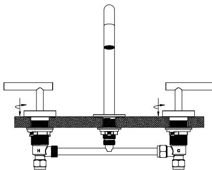
8. Slide the plates down to cover the fittings and tighten them in place.
