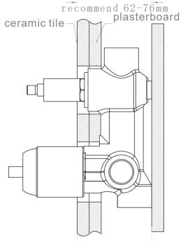
4. Remove the plastic sleeve and install sleeve of divertor.
