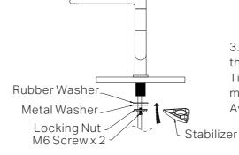
3. Install the rubber and metal washers, if a stabilizer is required, install the stabilizer after positioning the rubber washer.
