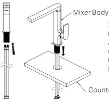
2. Attach the threaded tube to mixer body and screw the Pex hoses into the bottom of the mixer body.
