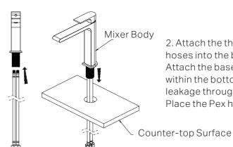
2. Attach the threaded tube to mixer body and screw the Pex hoses into the bottom of the mixer body.
