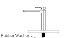
3. Install the rubber and metal washers, tighten the locking nut securely with the two M6 screws to ensure the mixer is firmly attached to the counter-top.
