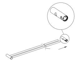
2. Use a hacksaw or pipe cutter to cut the towel rail to the desired length, then deburr the end with a file or grinder.
