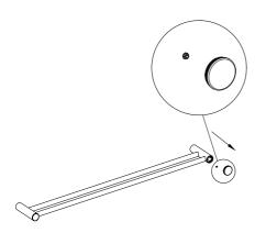
1. Detach the end cap from the right side of the towel rail. Loosen the grub screw holding the rail in place.
