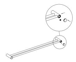
3. Insert the shortened rail back into the bracket. Tighten the grub screw to secure it, and replace the end cap.
