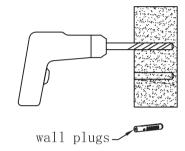
5. Drill pilot holes into wall stud approximately 60mm deep to suit mounting screws (and wall plugs if required).
