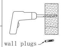
5. Drill pilot holes into wall stud approximately 60mm deep to suit mounting screws (and wall plugs if required).
