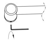
9. Tighten grub screws with allen key.
