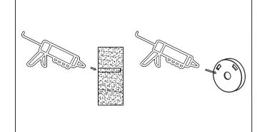
6. Apply small amount of silicon to mounting bracket and wall in and around the screw holes.
