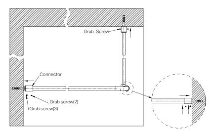
05. Confirm all connections are tight. Ensure the rail is stable and aligned.
