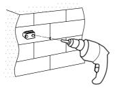
3. Use an electric drill with a 6mm drill bit to drill holes at the marked points.
