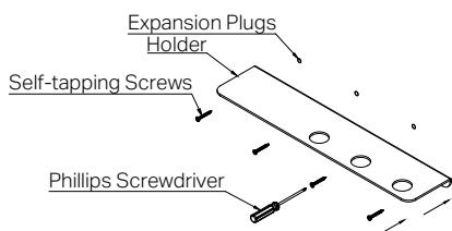
3. Align the holder with the holes and secure it with self-tapping screws supplied.
