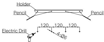
1. Drill four Ø6 mm holes, 120 mm centre to centre, at the marked location.
