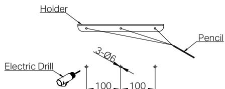
1. Drill three Ø6 mm holes, 100 mm centre to centre, at the marked location.
