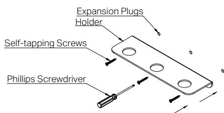
3. Align the holder with the holes and secure it with self-tapping screws supplied.
