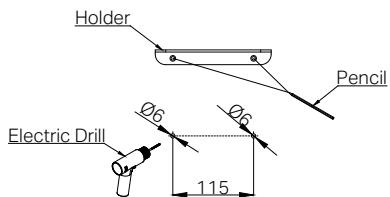
1. Drill two Ø6 mm holes, 115 mm centre to centre, at the marked location.
