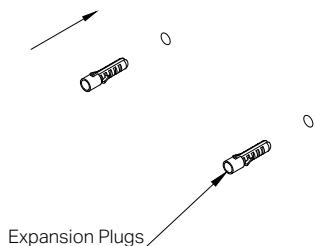
2. Place the supplied expansion plugs into both holes.
