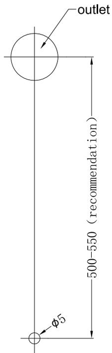
1. Drill a  $\phi 6$ mm hole at the outlet vertical downward position in the recommended range.
