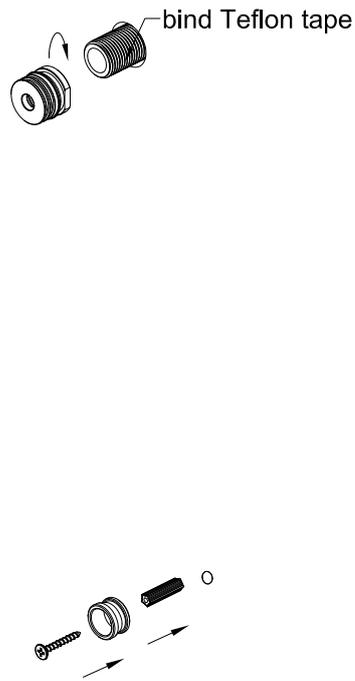
2. Screw the adapter on the outlet, and mount the bracket on the  $\phi 6$ mm hole by expansion plug and tapping screw.
